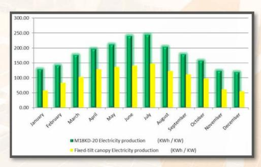
The \$368,000 investment in the solar trackers captured the 30% federal solar investment tax credit applicable on that year, with a resulting LCOE of 7 cents/kWh, compared with 24 cents/kWh under the ground mount fixed-tilt scenario. The resulting ROI is just 3.5 years Return On Investment (ROI) compared with an average seven to a 9 year ROI for fixed-tilt canopies.
